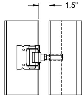
Gate hinge threads into the upper and lower inserts in the gate metal frame leaving about 1.5" from the edge of the gate to the gate post.
