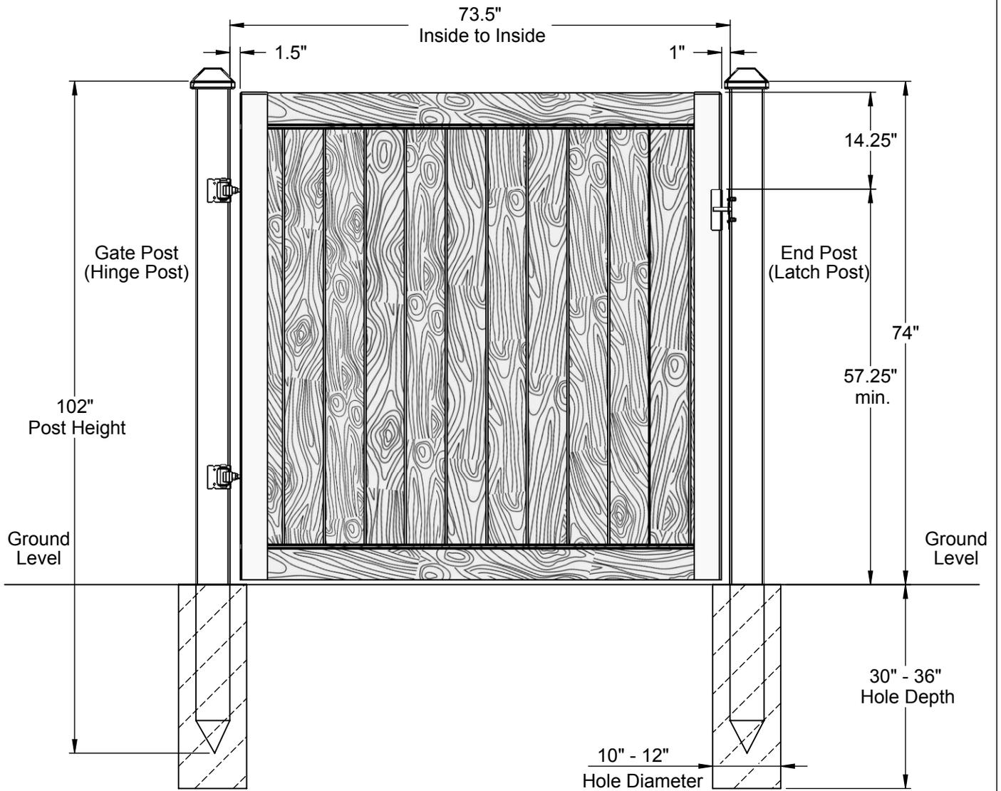
Gate is reinforced with a 1.5" galvanized steel box tube.
