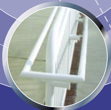
Wall mounted handrail can be fabricated on site using a mitre saw and our adjustable joiner to create a continuous configuration. Shown are two rail sections mitred to fit, including two internal joiners. They allow the rail to follow any wall and ramp configuration.
