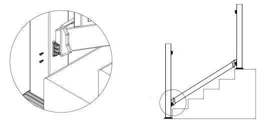
**Step 4 - Secure the bottom rail.** Attach the bottom rail to the nylon post brackets by using the (4)  $\#10 \times 1"$  pan-head screws. The bottom rail will be 1" off the step tread nosing with the rail inserted correctly into the nylon post brackets. Fasten two screws into each side of the nylon post bracket using the top and bottom slots of the nylon post brackets. Once secured, snap the 2" x 3-1/2" step bracket covers positioned in Step 3 onto the nylon post brackets.
