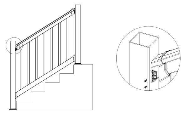
**Step 7 - Secure the top rail.** Position the top rail over the exposed ends of the balusters so that it is positioned on the resting flange of the installed nylon post brackets. Attach the top rail to the nylon post brackets by using the (4)  $\#10 \times 1"$  pan-head screws. Fasten two screws into each side of the nylon post bracket using the top and bottom slots of the nylon post brackets. Snap the alzar bracket covers positioned in Step 6 onto the nylon post brackets.
