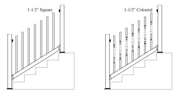
**Step 5 - Insert the balusters.** Having secured the bottom rail into place, insert the balusters into the bottom rail. If the 1-1/2" colonial balusters are being used make sure the balusters are inserted so the baluster tapers are uniformly installed.
