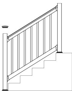
**Step 8 - Finish the section.** Secure the 4" x 4" post caps onto the post tops by applying PVC adhesive to the internal surfaces of the post caps. Set the caps onto the post tops. Wipe off any excess adhesive.
